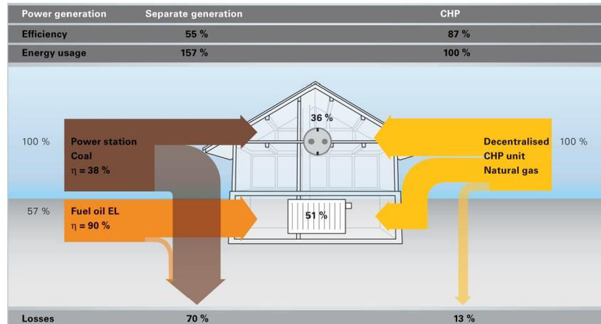
Fig. 3.9: Efficiency comparison of natural-gas-based CHP and separate generation of heat and electricity [Viessman, 2012].
