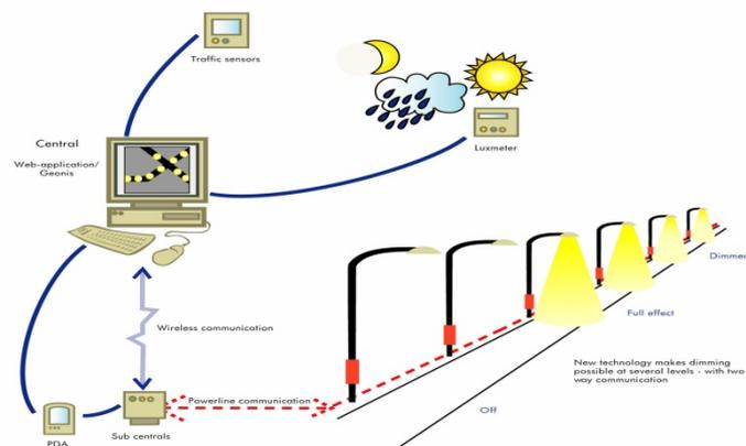
Fig. 4.2: Example on the intelligent road light control [CUD, 2008].
