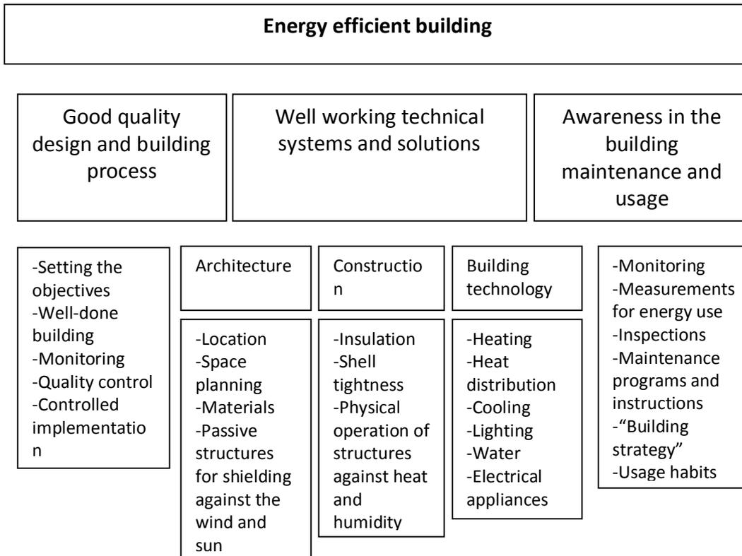
Fig. 5.1: Main factors in the realization of an energy efficient building.
