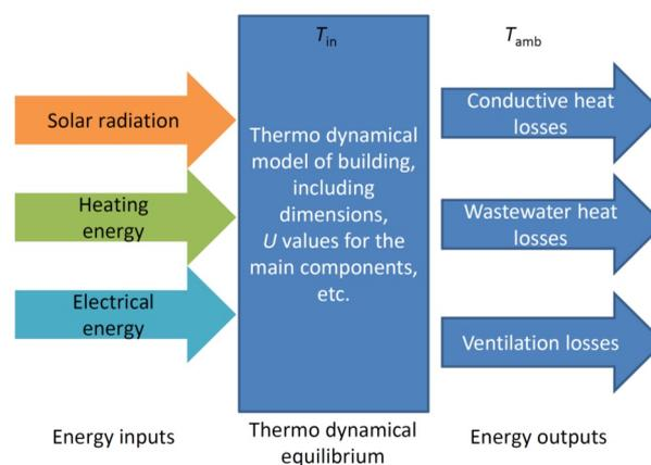
Fig. 6.1: Operational principle of the energy efficiency classification tool. It calculates the annual building heat energy consumption based on the given technical details of the building.
