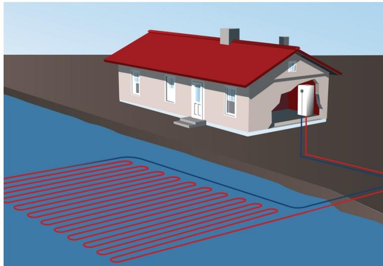
Fig. 3.6: Geothermal heat pump system requires installation of piping to the ground or for instance to the sea [IVT Nordic, 2012b].
