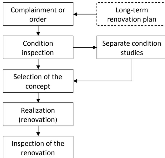
Fig. 2.5: Main flowchart of a renovation project [RIL 249-2009].
